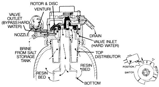
After fill, timer/switch action allows the motor to turn the rotor and disc into BRINING position. Water flow is directed to the nozzle. Suction, created by the nozzle and venturi, draws brine from the salt storage tank and injects it into the resin bed via the bottom distributor. Flow continues out the top distributor and to the drain. Hard water is available at the valve outlet.
