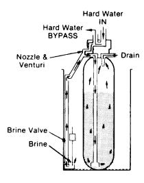
4 BACKWASH: During backwash, water flows UP through the resin tank (FIG. 7) at a fast rate to flush iron minerals, dirt and sediments from the bed and to the drain. The bed lifts and expands for good cleaning.
