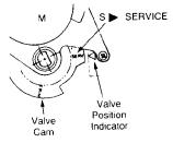
Use the MANUAL ADVANCE procedures, page 23. With the RECHARGE NOW button, advance through the recharge cycles until the valve stops in service position, and RECHARGE no longer flashes in the timer.
