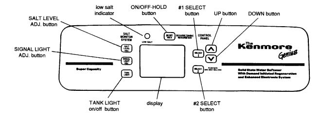
When the transformer is plugged in, the model code AR31, and a test number (example: A1.0) show in the face plate display for 4 seconds. Then, 12:00 AM and PRESENT TIME begin to flash.
