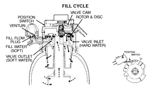
To begin a regeneration, the electroic timer energizes the circuit to the valve motor. The valve motor rotates the rotor and disc and the valve cam until the position switch lever drops, to open the motor circuit and position the valve in FILL. As the rotor and disc rotates, the port opens for SOFT water fill through the venturi. Fill flow continues to the brine valve, and into the salt storage tank. Soft water is still available to the house lines.
