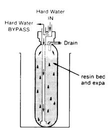
5 FAST RINSE: Backwash is followed by a fast flow of water down through the resin tank. The fast flow packs the resin bed and gets it ready for return to service (FIG. 8).
