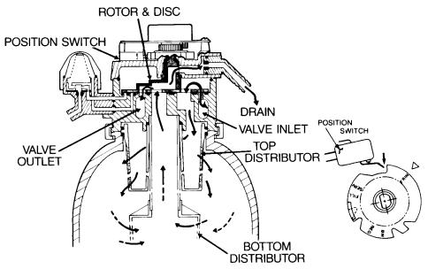
During FAST RINSE, the rotor & disc is positioned so water flow enters the resin tank through the top distributor, and exits through the bottom distributor, to the drain.
