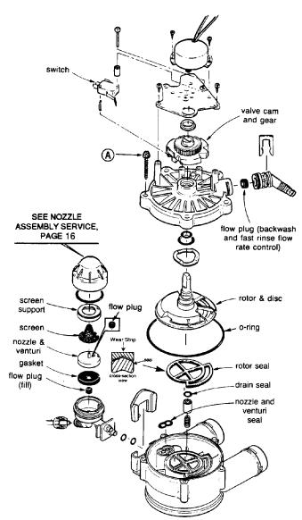
Lubricate the gear on the motor, and the valve cam gear with Molykote grease, or other high quality gear lubricant.
