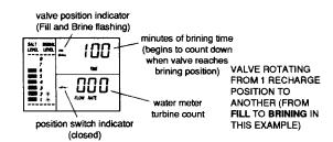
All of the preceeding displays show what position the valve is in, if the turbine is operating, and the position switch open or closed status.
