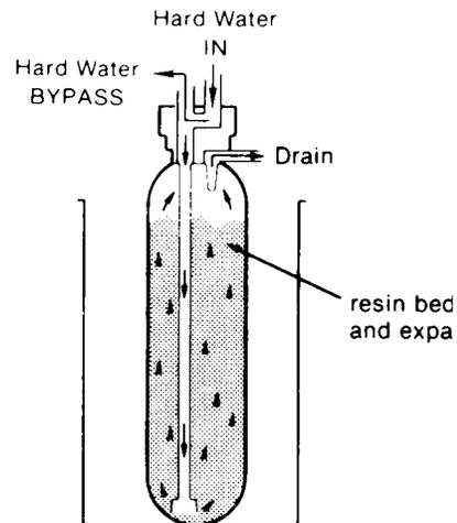
**5] FAST RINSE:** Backwash is followed by a fast flow of water down through the resin tank. The fast flow packs the resin bed and gets it ready for return to service (FIG. 8).
