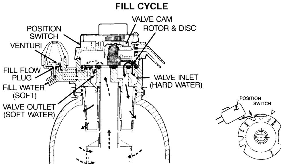
To begin a regeneration, the electroic timer energizes the circuit to the valve motor. The valve motor rotates the rotor and disc and the valve cam until the position switch lever drops, to open the motor circuit and position the valve in FILL. As the rotor and disc rotates, the port opens for SOFT water fill through the venturi. Fill flow continues to the brine valve, and into the salt storage tank. Soft water is still available to the house lines.
