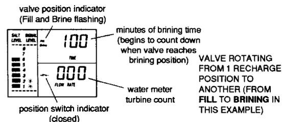
All of the preceding displays show what position the valve is in, if the turbine is operating, and the position switch open or closed status.
