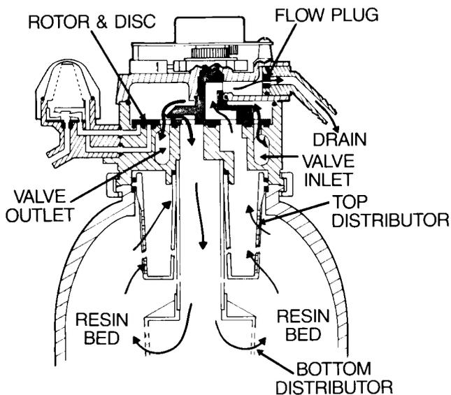
Timer/switch action again allows the motor to turn the rotor & disc to place the valve in BACKWASH, stopping water flow to the nozzle. Water is routed down and out the bottom distributor, up through the bed, and out the top distributor to the drain. The fast flow (controlled by a flow plug in the drain fitting) flushes dirt, sediments, iron deposits, remaining brine and hardness to the drain.
