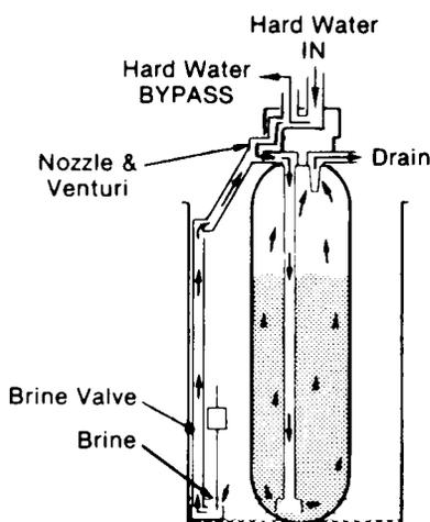
**4] BACKWASH:** During backwash, water flows UP through the resin tank (FIG. 7) at a fast rate to flush iron minerals, dirt and sediments from the bed and to the drain. The bed lifts and expands for good cleaning.
